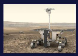
First ESA rover, will analyze soil samples digging 2 meters deep
