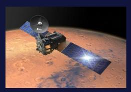
TGO orbits Mars searching for trace gases (methane)
